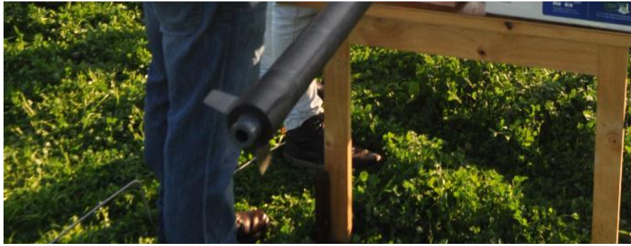
Figure 2 PVC water rocket nozzle and carbon fibre fins
