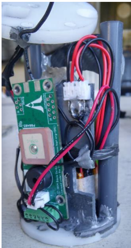
Figure 3 Partially assembled payload frame for test rocket was made from plastic and carbon fibre. Based on this design a carbon fibre frame was made for Ascension III. Pictured is the Altus Metrum TeleMetrum altimeter.
