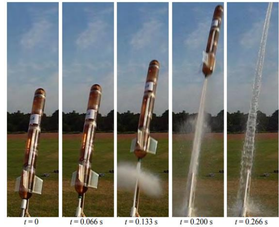
Figure 1.4-1: Video analysis of a water rocket at launch (De Podesta, 2006)
