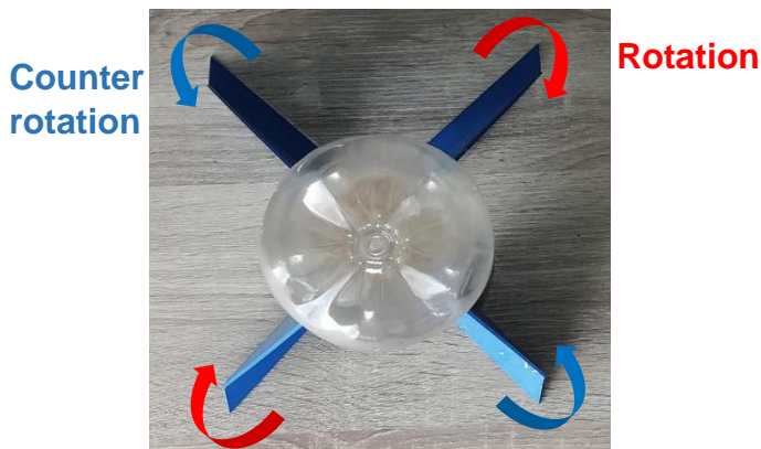
Figure 2.4-3: Top view of Ctrl displaying the disposition of the fins
