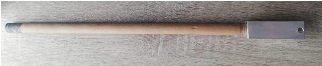
Figure 4.3-2: Aluminium link and wooden axle for the test rig
