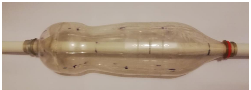
Figure 4.2-1: Fuselage for the wind tunnel test rig
